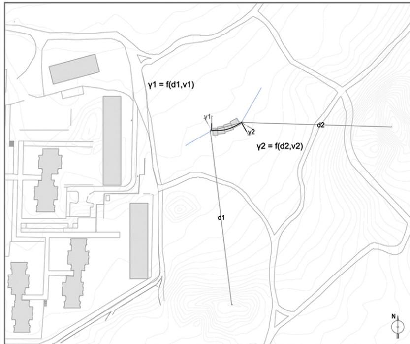
Fig. 11. Association of the summer and winter wind velocity vectors and the adjacent hills' distances with the tangent directions of the base curve.
