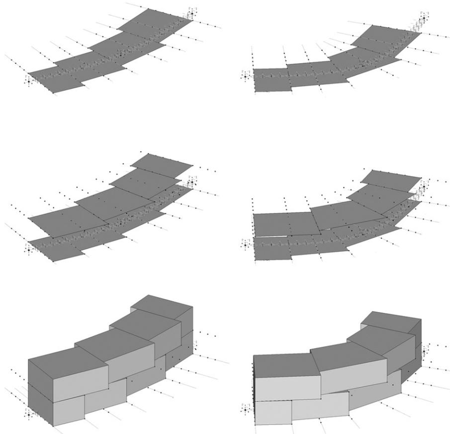
Fig. 13. Algorithmic steps of the building core feature for two different base curve cases.
