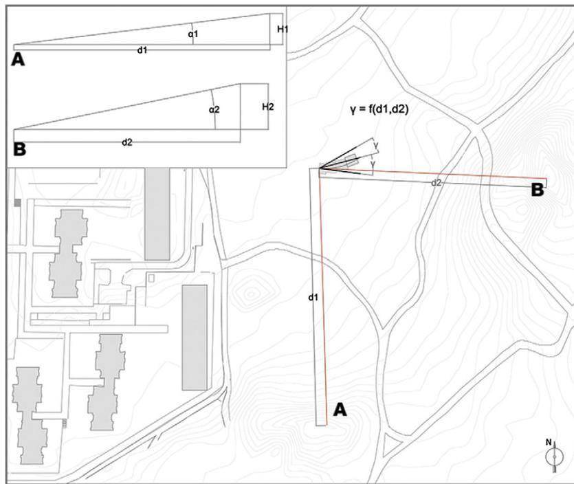
Fig. 12. Association of the optimum orientation with the adjacent hills to ensure maximum insolation.
