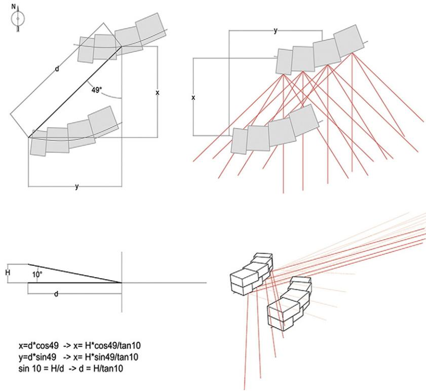
Fig. 10. Building proximity study to ensure maximum solar insolation during the underheated period.
