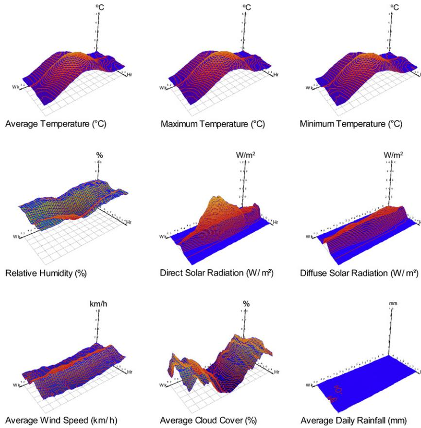
Fig. 2. Prevailing climatic conditions at the University of Patras site—Annual plots per week and hour of day of average, maximum and minimum temperature, relative humidity, direct and diffuse radiation, wind speed, cloud cover and rainfall.
