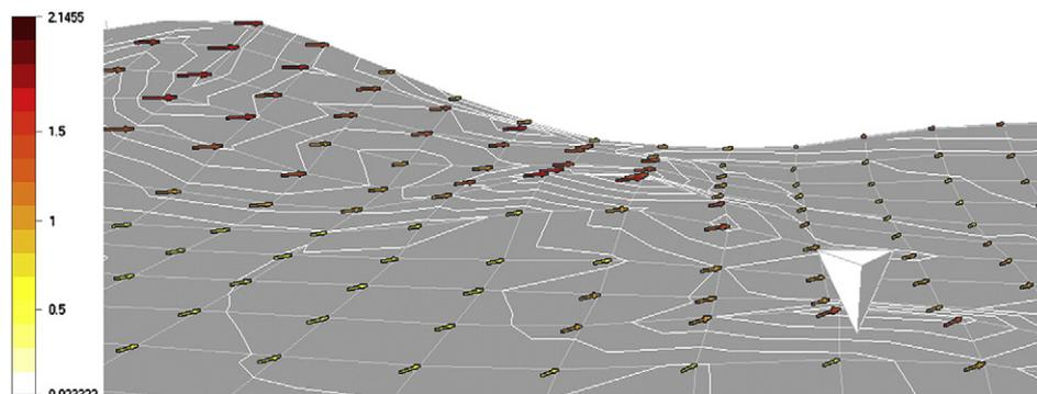
Fig. 7. Wind velocity vector field at 5 m above ground level generated by the CFD simulation for the University of Patras campus.
