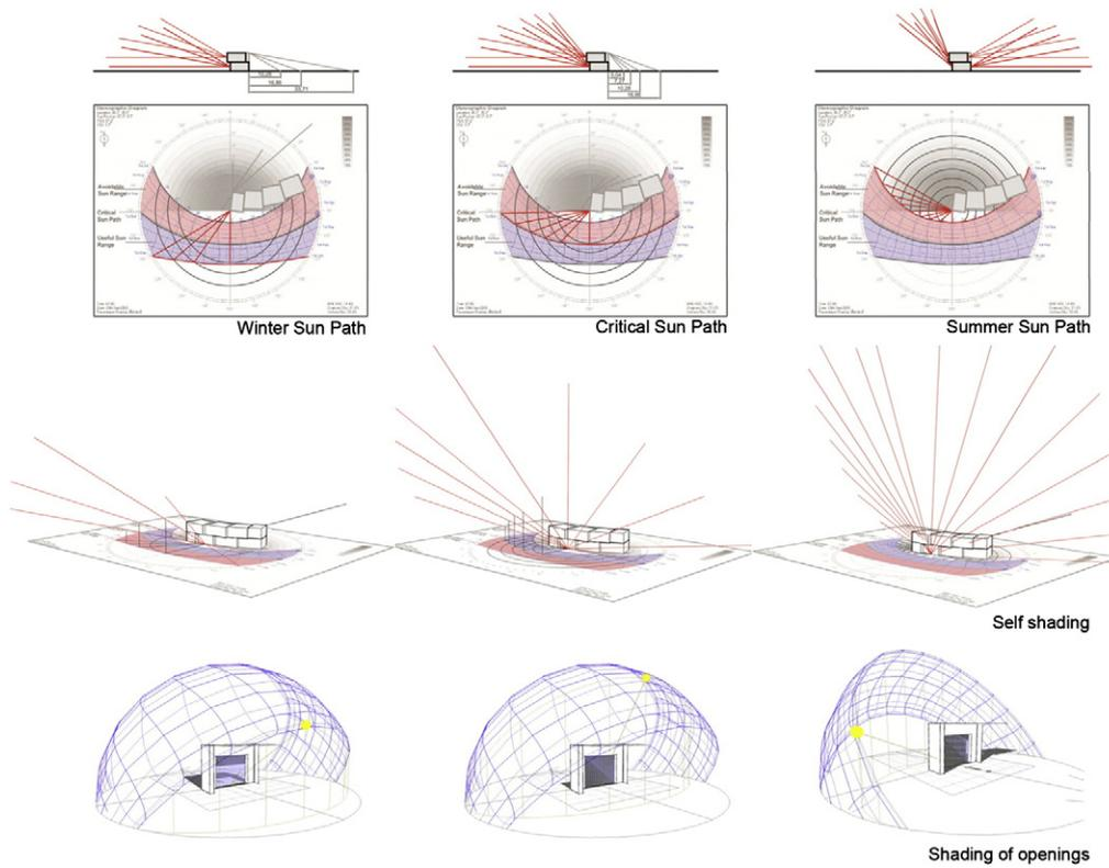
Fig. 8. Self shading study of the basic building geometry, its deformation and its openings for the winter and summer solstice and the critical sun path.
