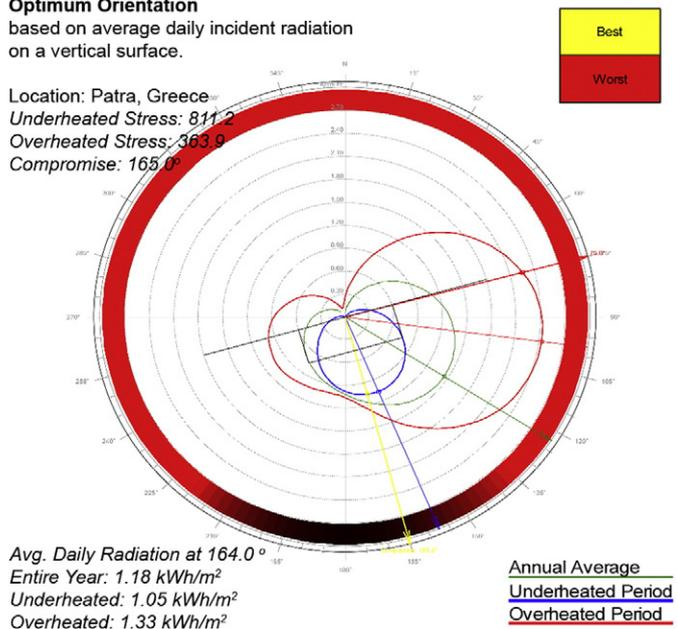
Fig. 9. Optimum orientation based on an annual calculation of solar gains in relation to thermal comfort, generated by the Ecotect Weather Tool.
