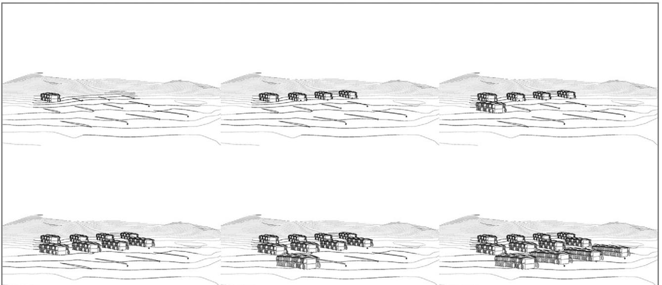
Fig. 15. An arrangement of building modules on the University of Patras site generated hierarchically by the site geometry algorithm.
