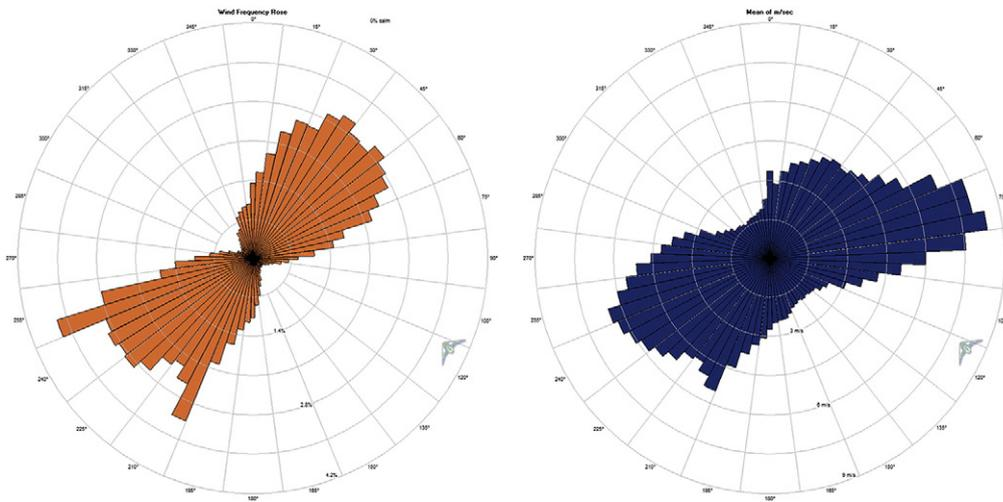
Fig. 4. Wind frequency graphs generated by the meteorological data for the University of Patras Campus—Wind frequency and mean velocity per direction.
