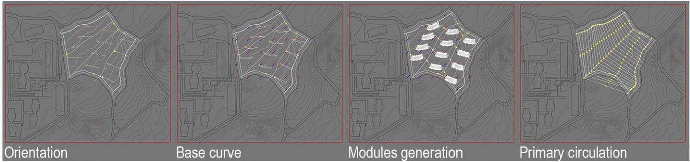
Fig. 16. Sequence of the generation of building modules on the University of Patras campus by the site geometry algorithm.
