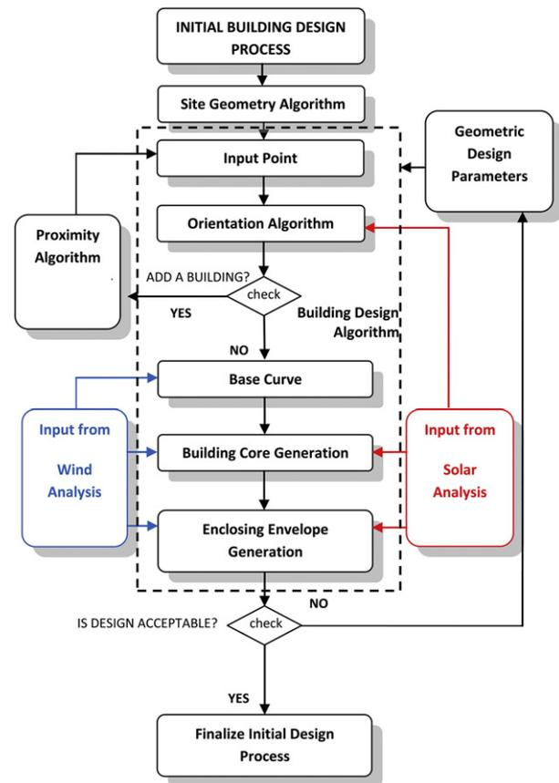
Fig. 1. Flow-chart of the proposed parametric design methodology.
