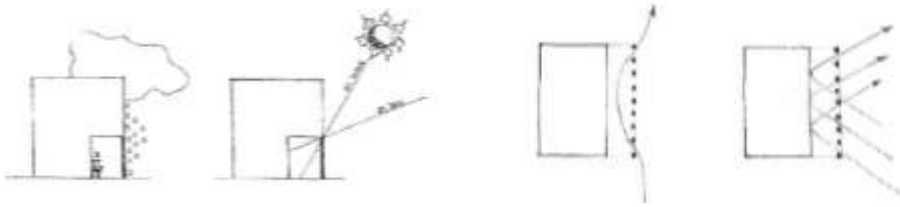
Figure 4 Portico: Diagrammatic sections, winter rainfall and winter and summer penetration and diagrammatic plans, wind flow blowing parallel to the open surfaces, laminar flow and at an angle, turbulent flow
